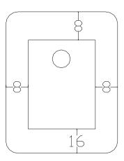
FIGURE 3 - CLEARANCE TO COMBUSTIBLES (Top View)
