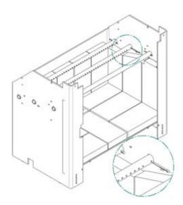
Figure 4.5 – Secondary Air Tube Replacement
