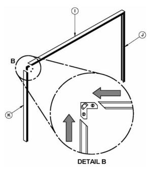
Insert the superimposed brackets (F) and (G) with the screws (H) in the groove of each decorative trim (I), (J) and (K) (see **DETAIL B**). Align the corners of the angled side of each trim, and then tighten the screws (H) to secure the trims.
