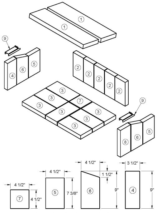
Figure 4.4b – Firebrick layout for CW2500
