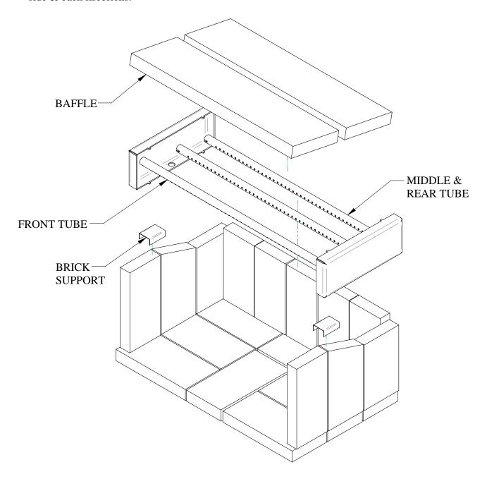
Figure 4.4a – Baffle installation & removal for CW2500
