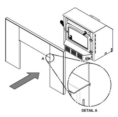
Once the faceplate is assembled, align the notches, located at the top of each side of the faceplate opening, with the top of the insert and slide the assembly toward the front of the insert (see **DETAIL A**).
