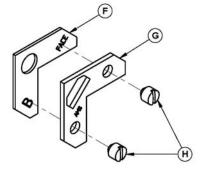
Partially thread the screws (H) on the trim's corner bracket (G) then superimpose the corner brackets (F) and (G) as shown in the image on the left.
