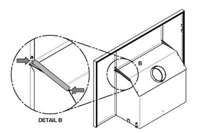
Center the insert into the fireplace opening. Adjust its height using the leveling bolts on each side of the convection air jacket box until the faceplate is properly seated on the floor of the hearth extension.
