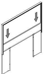
Align the trim assembly with the left and right edge of the faceplate and slowly slide it down over the faceplate.
