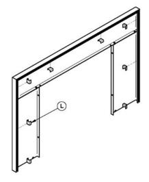
Secure the trim to the faceplate by squeezing the eight trim retainers (L) between the inner edge of the trim and the front of the faceplate. As in the image on the left.
