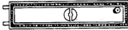
Fig. G-5 Ash Door 43" (Extra Large), 36" (Large), 29" (Small) – 7/16 fiberglass Seals ash door to front.
