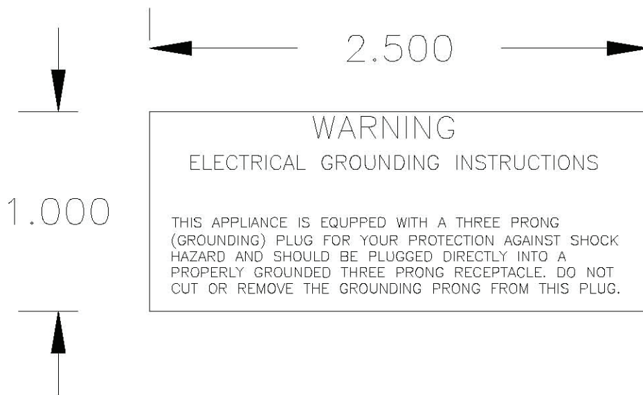
FIGURE 27: WARNING LABEL PROPER ELECTRICAL GROUND
