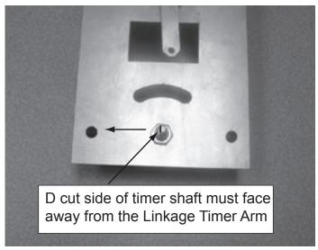
Figure 4.22 D Cut on Shaft
