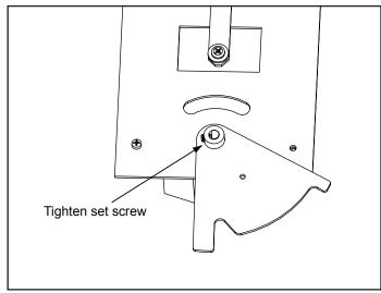
Figure 4.23 Linkage Control Arm Installed
