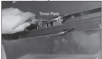
Figure 4.16 Remove Screws from Timer Mounting Plate
