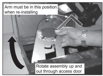
Figure 4.18 Removing Timer Assembly
