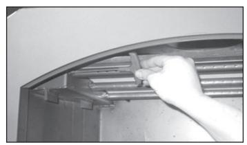
Figure 4.6 Removing Manifold Tube
