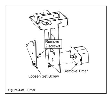
Install new timer using same two screws. It is very important that the D cut side of the timer shaft is facing the opposite side of the linkage timer arm. See Figure 4.22.
