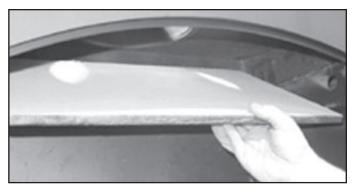
Figure 4.7 Removing Baffle (shown without ceramic blanket)
