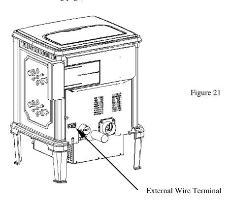
The external Thermostat wire terminal has been pre-wired to the thermostat wire Terminal on the back of the control board (See figure 21)
