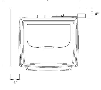
Figure 12 (Top View) Clearances Sides and Back
