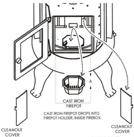
LEFT CLEANOUT COVER AND RIGHT CLEANOUT COVER INSTALL INTO BACK WALL OF FIREBOX, USING THE HOOKS ON THE BACK EDGES OF THE COVERS.
