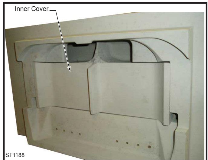
Fig. 29 Remove inner cover.
