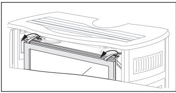
Figure 3.20 - Release the latches to remove the glass frame.
