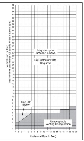
Figure 2.7 - Horizontal vent termination window.
