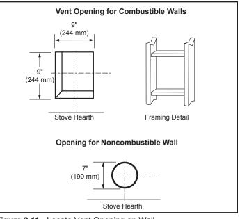
Figure 3.11 - Locate Vent Opening on Wall
