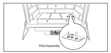
Figure 4.1 - Pilot Assembly location.
