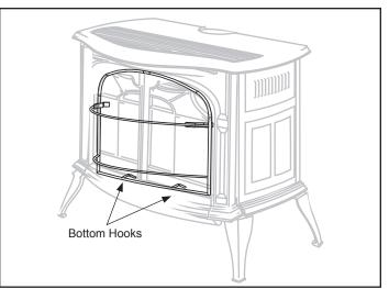
Figure 3.27 - Install safety barrier screen.
