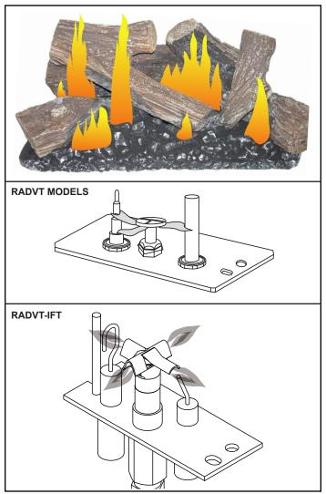
Figure 4.2 - Correct pilot and burner flame appearance.
