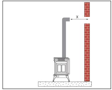
Figure 3.13 - Horizontal Length Requirement
