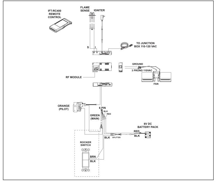
Figure 6.3 - RADVT-IFT Wiring Diagram
