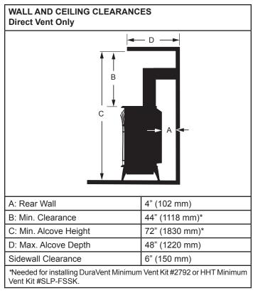
Figure 2.6 - Dimensions and clearances to ceiling or alcove.
