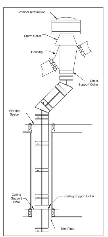
Figure 3.17 - Typical Vertical Venting Configuration
