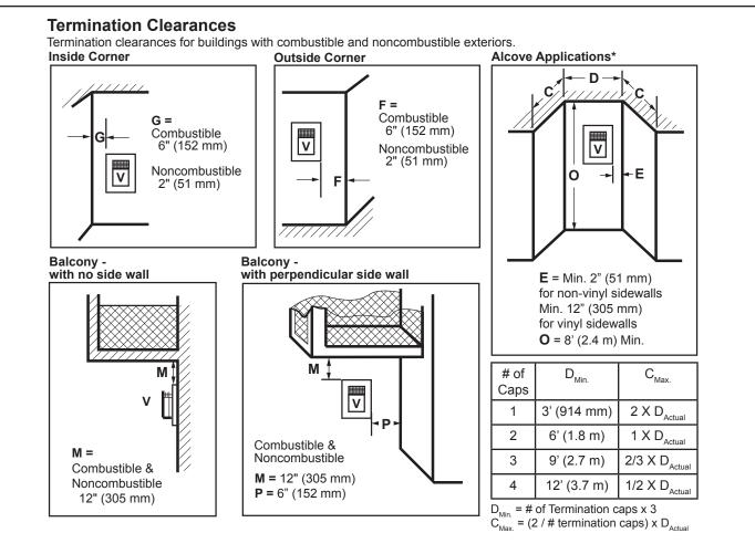
\*NOTE: Termination in an alcove space (spaces open only on one side and with an overhang) is permitted with the dimensions specified for vinyl or non-vinyl siding and soffits.
