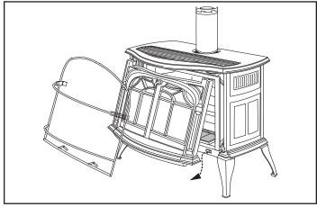
Figure 3.19 - Remove the safety barrier and stove front.
