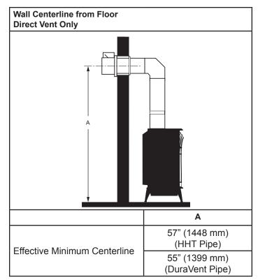
Figure 2.5 - Minimum wall centerline.
