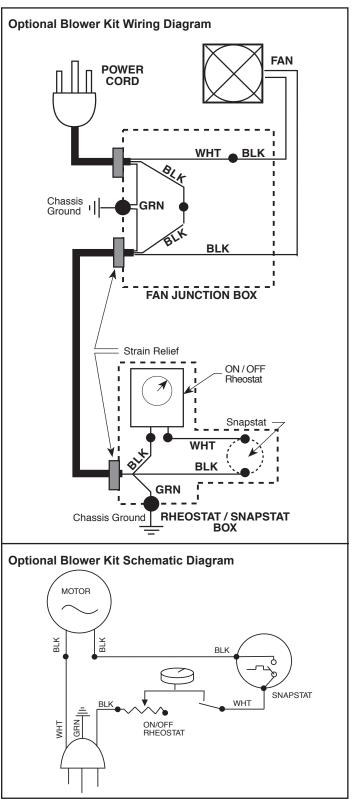
Figure 6.2 - Fan circuit.
