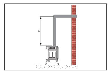
Figure 3.12 - Vertical Height Requirements
