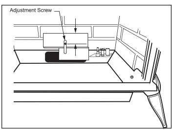
Figure 2.9 - Loosen screw to adjust restrictor plate.
