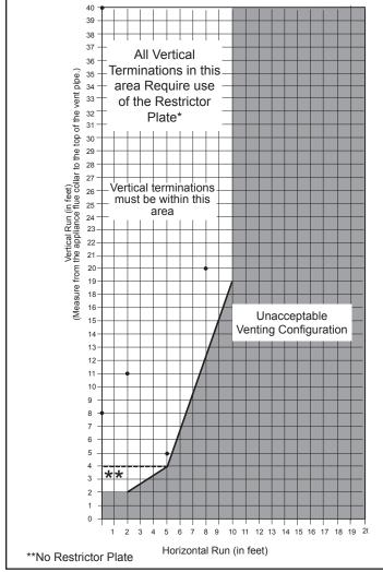
Figure 2.8 - Vertical vent termination window.
