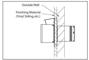
Figure 3.1 - Termination cap on wall
