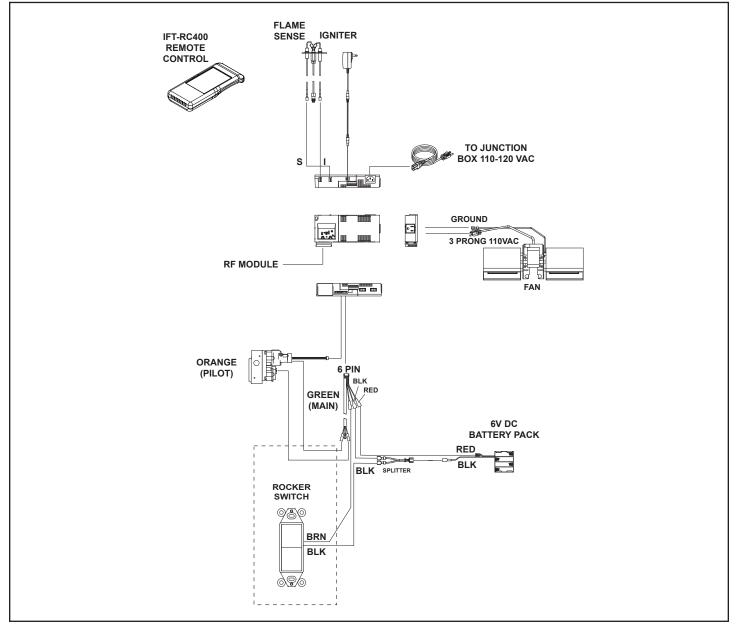
Figure 3.26 - RADVT-IFT Wiring Diagram
