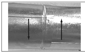
Figure 3.8 - Rotate Seams for Disassembly
