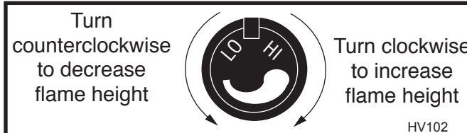
Fig. 34 Flame adjustment knob for Honeywell valve.
