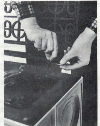
Insert loose pin into hinge and receptacle as shown. Tap in with hammer. With grille raised, carefully slide on the top tile section.
