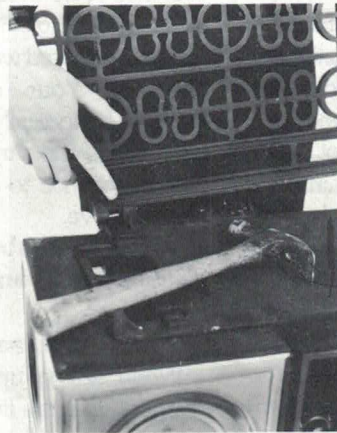
To attach top grille, insert pin affixed to grille into its metal receptacle on stove top to form one hinge. Tap it lightly with a hammer to secure it.
