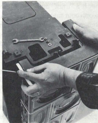
Insert top bolt in slot. Be sure tile frame fits securely and is lowered as far as it will go. Tighten top nuts with wrench provided (not too tightly!).
