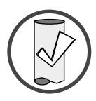
Inspect the chimney connector and chimney at least twice monthly and clean if necessary. Creosote may build up and cause a house fire.
