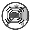
Overfiring the appliance may cause a house fire. If a unit or chimney connector glows, you are overfiring.
