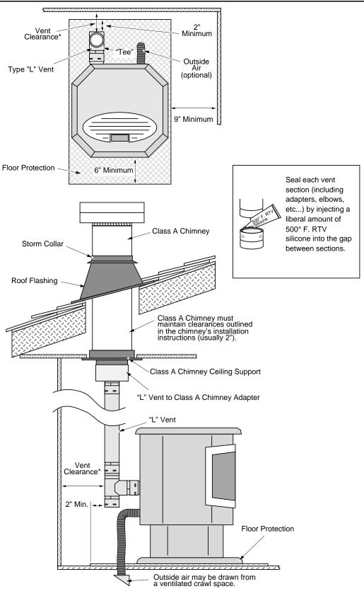
\* Install vent at clearance specified by the vent manufacturer.
