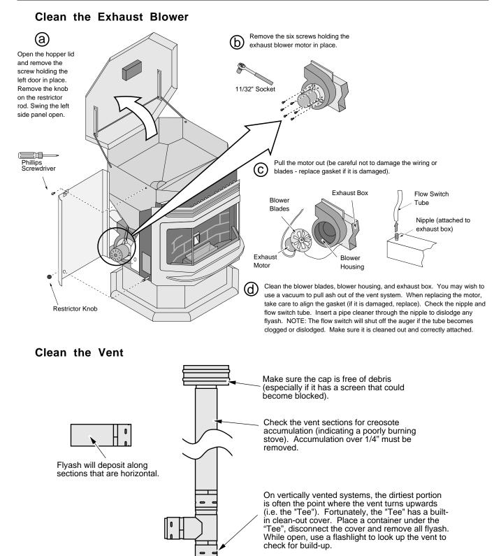
Warning: Whenever any portion of the pellet vent is disconnected, the joints must be sealed with RTV 500° F. silicone sealant.
