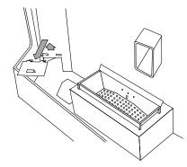
(d) Slide the ash pan trap door forward to expose the ash dumps (the door can be removed and cleaned if necessary)
