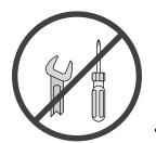
Never remove, replace, modify or substitute any part of the heater unless instructions are given in this manual. All other work must be done by a trained technician. Don't modify or replace orifices.
