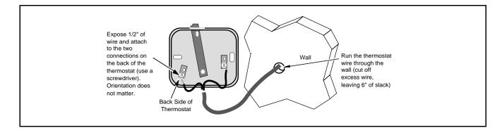
4 Pull the cover off the thermostat. Place the thermostat in location and attach it to the wall through the two obround holes (use the appropriate screws for the type of wall it is being attached to). Replace the cover on the thermostat to complete the installation.
