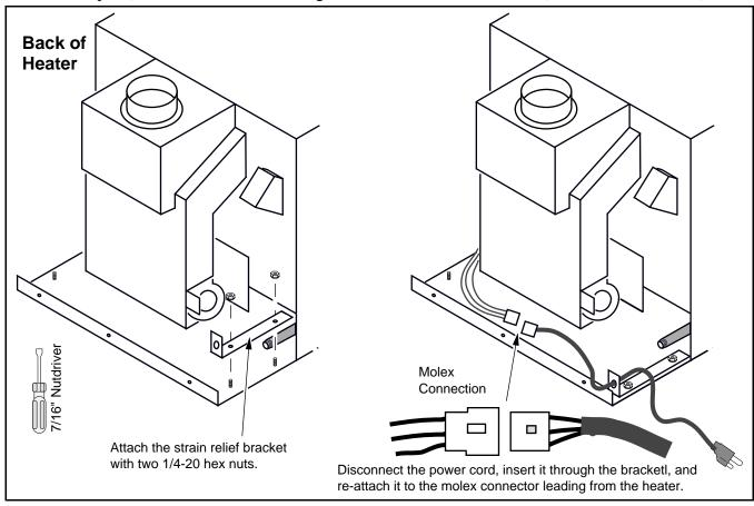
Pull gently on the power cord to take out any extra slack. Attach the strain relief (it is shipped attached to the power cord - see the illustration below).
