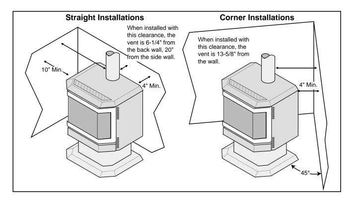
+ Clearances may be reduced by methods specified in NFPA 211, listed wall shields, pipe shields, or other means approved by local building or fire officials.
