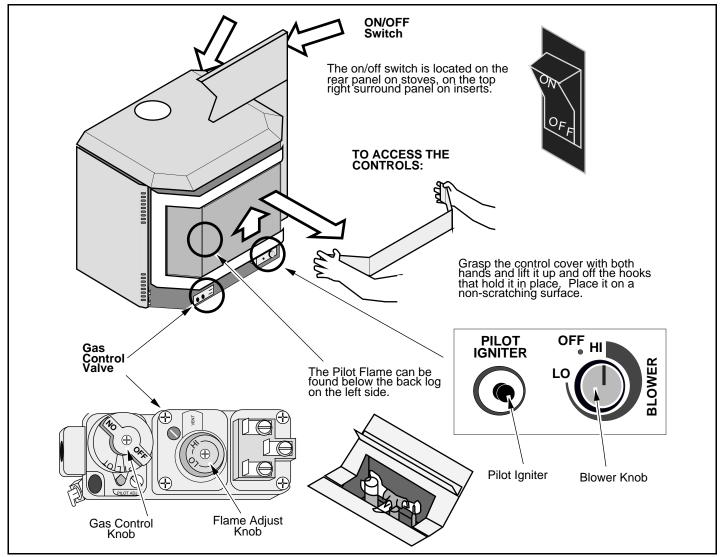
**Blower Knob** This knob controls the speed of the internal convection blower that pushes the
