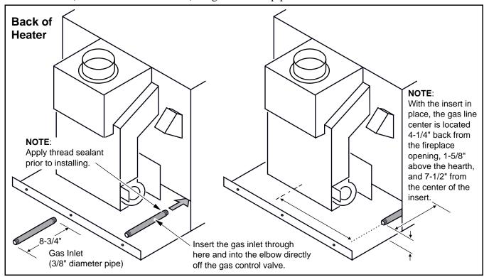
! Leak check all gas line connections.
