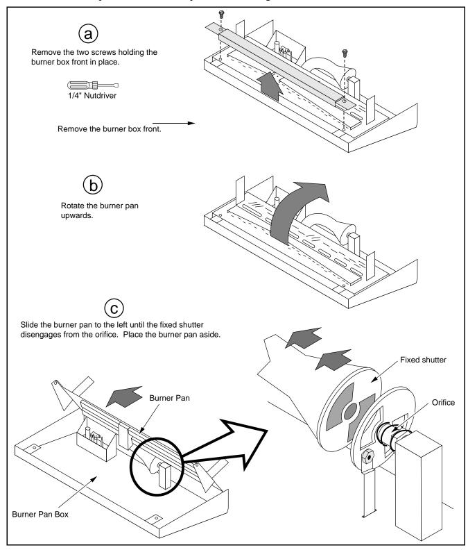
4 Follow the directions below to remove the natural gas orifice. Apply thread sealant to the LP orifice (#49 - it has "49" stamped on it) and tighten in place with a 1/2" open end wrench. Replace the spring. Slide the adjustable shutter back in place.
