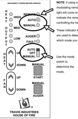
modulating remote, this light will come on to indicate the remote is controlling the heater.
