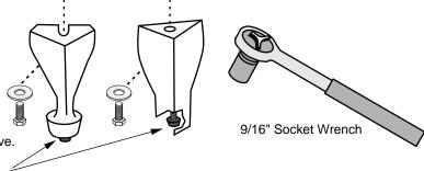
These rubber-tipped bolts are for leveling the stove. Make sure they contact the floor. Do not adjust with weight on the legs, the rubber tips may tear.
