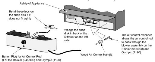
3. Make sure the wires leading to the snap disk are routed above the left side blower outlet (to prevent damage to the wires during installation). Install the blower following the directions below.
