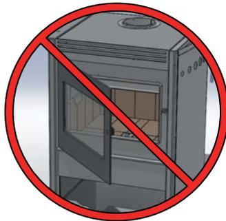
Never burn the stove with the loading door open. Leaving the door cracked open may damage the combustor.
