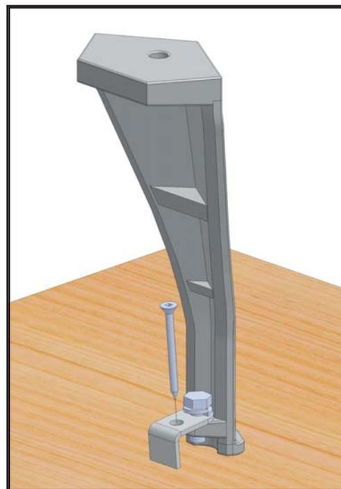
**In mobile home installations, the stove must be securely fastened to the floor using the tie-downs provided in the outside air kit. Use the leg anchor kit (Z2872) to secure stove to floor. ALSO, a #8 ground wire must be attached to the stove and an appropriate ground.**
