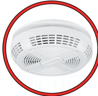
Install at least one smoke detector on each floor of your home to ensure your safety. It should be located away from the woodstove and close to the sleeping areas. Locating a smoke detector too close to a woodstove can cause the smoke detector alarm to sound if a puff of smoke is emitted while the woodstove door is open during reloading. Follow the smoke detector manufacturers placement, installation, and maintenance instructions.
