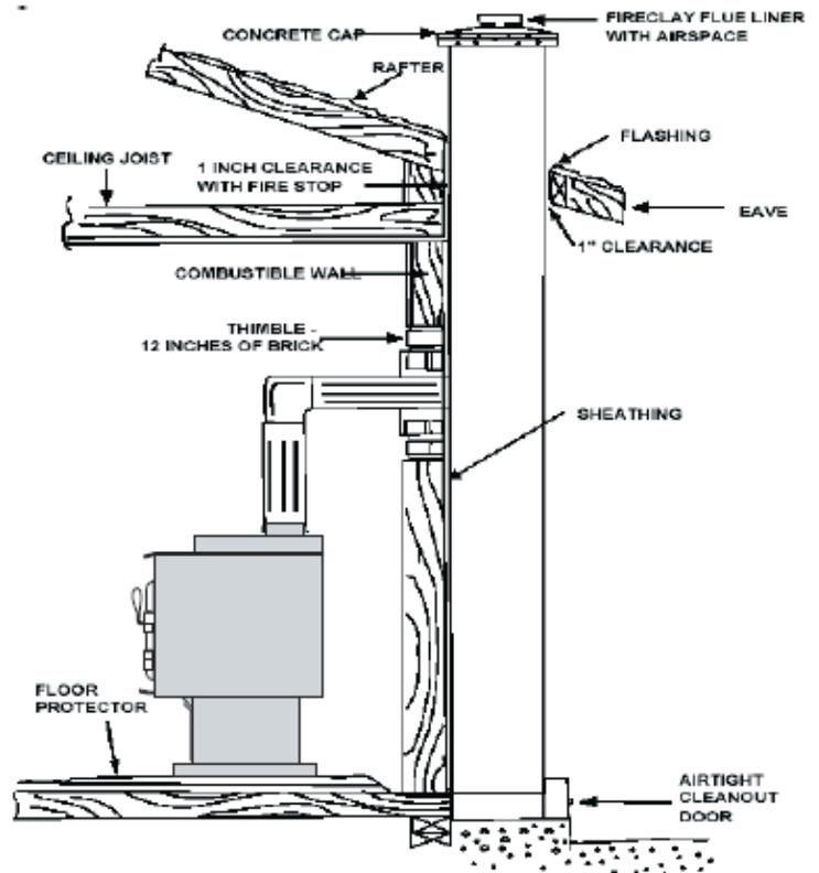
Your local dealer or local jurisdiction can provide details of approved methods of passing a chimney connector through a combustible wall in your area. In USA, the National Fire Protection Association has minimum standards to comply with. In Canada, this type of installation must conform to CAN/CSA-B365, Installation Code for Solid Fuel Burning Appliances and Equipment.
