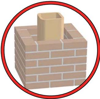
This appliance must be connected to a listed high temperature (**ULC629 IN CANADA OR UL-103HT IN THE USA**) residential type factory build solid fuel chimney or an approved masonry chimney with a flue liner.
