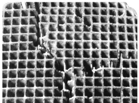
**PROBLEM - MECHANICAL CRACKING**
