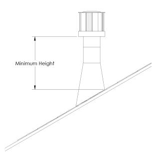
To prevent water seepage install the flashing with upper portion slid under the roofing material and the lower portion over the roofing material.
