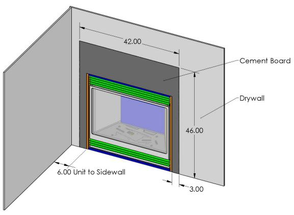
**Figure 3C Cement Board Dimensions**
