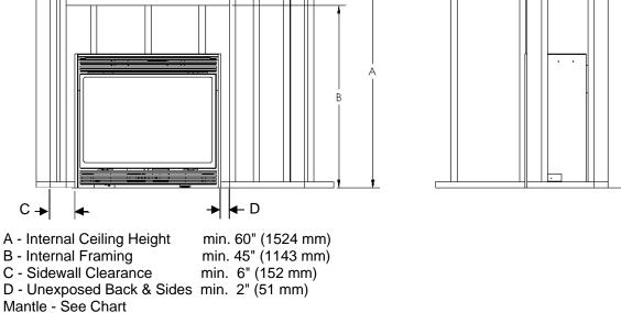
Vertical Vent - 1" (25 mm) to outside surface Horizontal Vent - 1" (25 mm) to outside bottom & side surface, 2" (51 mm) to outside top surface Can be installed on a combustible surface.
