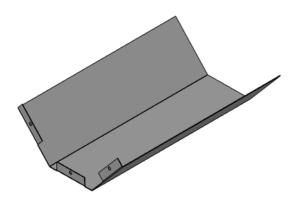
The heat shield which comes with the appliance, needs to be mounted vertically on top of the appliance. The three holes line up with the ones on top of the appliance, in front of the flue collar. Use three screws to mount the heat shield.
