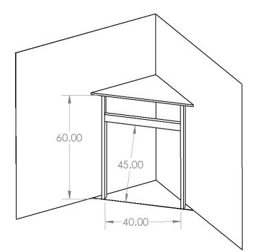
Figure 3C Minimum Framing Dimensions
