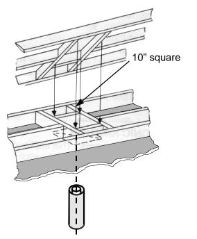
Use a suitable round or square support through the roof. Ensure adequate heat shield protection is provided.
