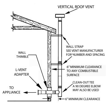
Locate terminations: a) not less than 3 feet above any forced air inlet located within 10 feet; b) not less than 4 feet below 7. Termination should not be located so that hot exhaust or horizontally from, or one foot above, any door, window or gravity air inlet into any building; c) not less than two feet from an adjacent building and not less than 7 feet above grade when located adjacent to a public walkway. Mobile home in-
