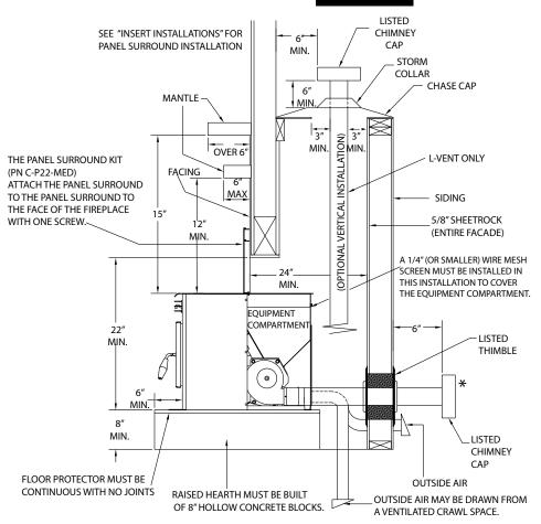
\* IF CHOOSING TO VENT HORIZONTALLY THROUGH THE WALL, WE RECOMMEND TERMINATING VERTICALLY WITH AN ADDITIONAL RUN OF AT LEAST 5 FEET.
