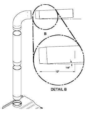
FIGURE 2.3 (B) Minimum Slope
