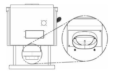
2- Locate the centre of the pedestal base on the floor and cut a 5 1/2" X 5 1/2" (140 mm X 140 mm) hole in the floor under the unit. Centre the unit over the hole.
