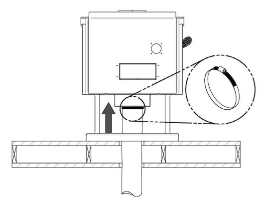
4- On the lower level, cut a 5 1/2" X 5 1/2" (140 mm X 140 mm) hole into the wall chosen to install the air intake. If there is a vapor barrier, attach the flaps around the opening. Insert the flexible pipe into the hole and secure it to the fresh air intake with the second adjustable collar. Secure the air intake finishing cap on the outside wall using 4 screws (not provided) and seal its border to prevent water infiltration.
