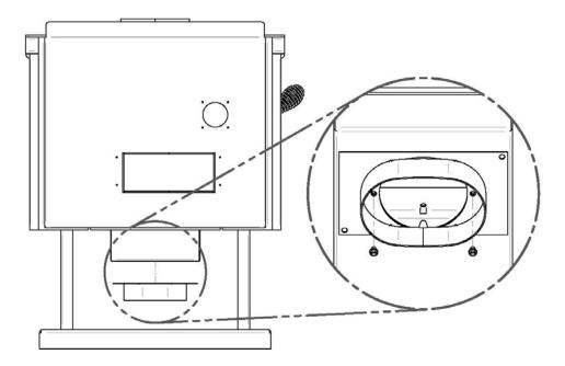
2- Insert the flexible pipe through the opening behind the base of the unit to connect to the adapter under the firebox and secure it with a adjustable collar.
