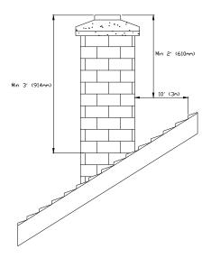
FIGURE 2.2 Minimum Height of the Chimney
