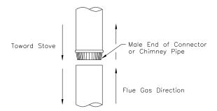
FIGURE 2.3 (A) Connecting Sections
