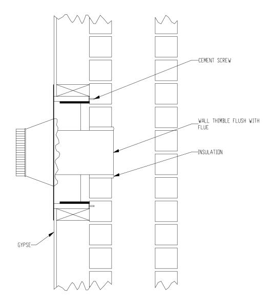
FIGURE 2.2.2 (B) Factory Built Thimble
