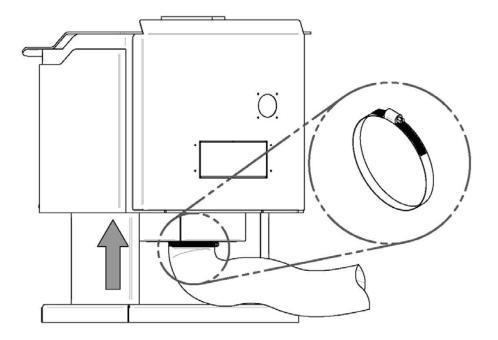
3- Cut a 5 1/2" X 5 1/2" (140 mm X 140 mm) hole into the wall chosen to install the air intake. If there is a vapor barrier, attach the flaps around the opening. Insert the flexible pipe into the hole and secure it to the fresh air intake with the second adjustable collar. Secure the air intake finishing cap on the outside wall using 4 screws (not provided) and seal its border to prevent infiltration of water.
