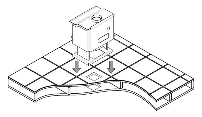
3- Pull the insulated flexible pipe from beneath the floor up to the 5" adapter. Secure the insulated flexible pipe to the 5" adapter with an adjustable collar.
