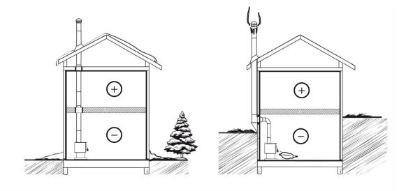
Good System Design Inside chimneys are preferred because even when no fire is burning, there is normally upward flow in the system. Inferior System Design Outside chimneys are a problem because when no fire burns they will go into cold backdraft if the stove is installed low in the house.
