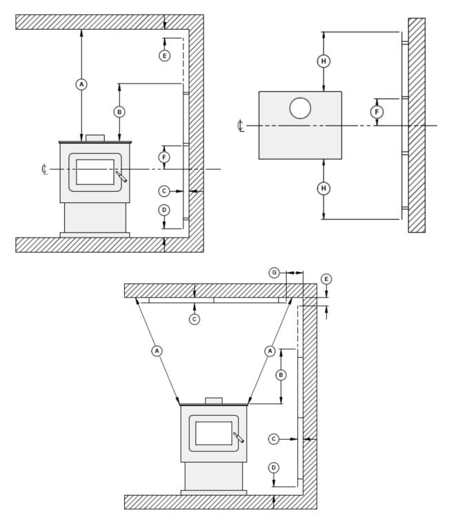
**Clearances for shield construction**
