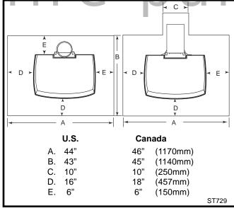
Fig. 11 Required floor protection dimensions.
