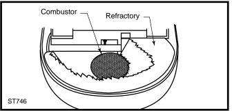
Fig. 33 A cutaway view of the combustor and its refractory cover. 2006063
