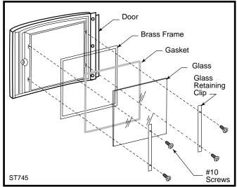
**Fig. 31** In order of assembly, the front door glass components include a brass frame, gasket, glass, two clips and four screws.
