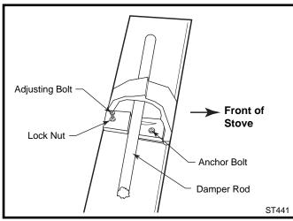
Fig. 32 Damper adjustment.
