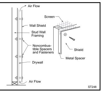
Fig. 13 Approved wall shield construction.
