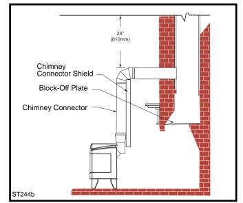
**Fig. 7** The connector enters flue above the fireplace. If the clearance between the chimney connector and either the mantel and/or the ceiling is inadequate, special protective shields will be required.
