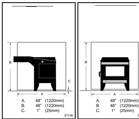
**Fig. 19** Side wall shield dimensions for a rear exit installation.
