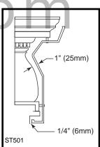
**Fig. 14** A custom-formed mantel shield.
