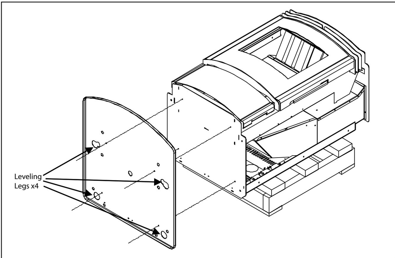
Figure 5: Installing Hearth Pad Pedestal onto EF5.
