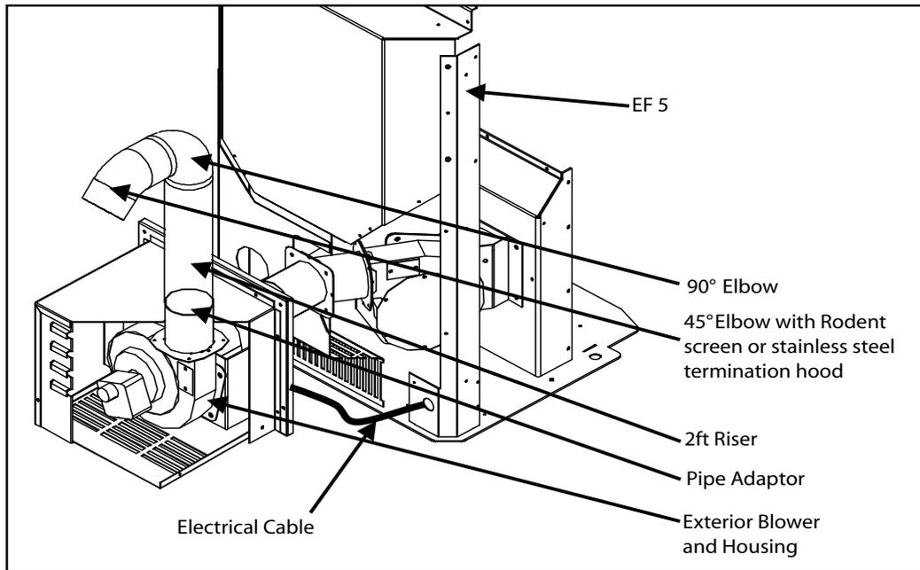
Figure 20: Through Wall Installation with Exterior Blower Kit.
