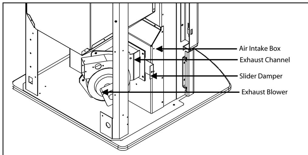
Figure 26: Slider/Damper Plate in Unit.
