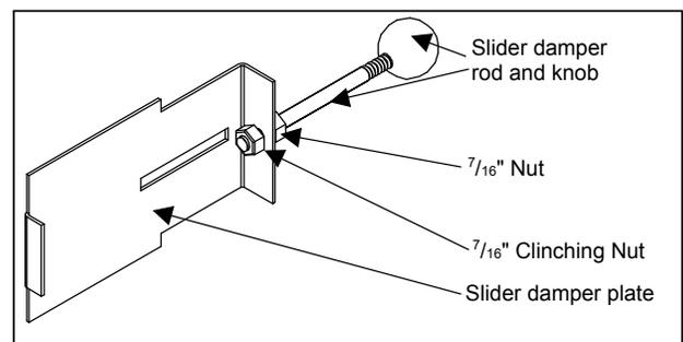
Figure 24: Slider/Damper Assembly.
