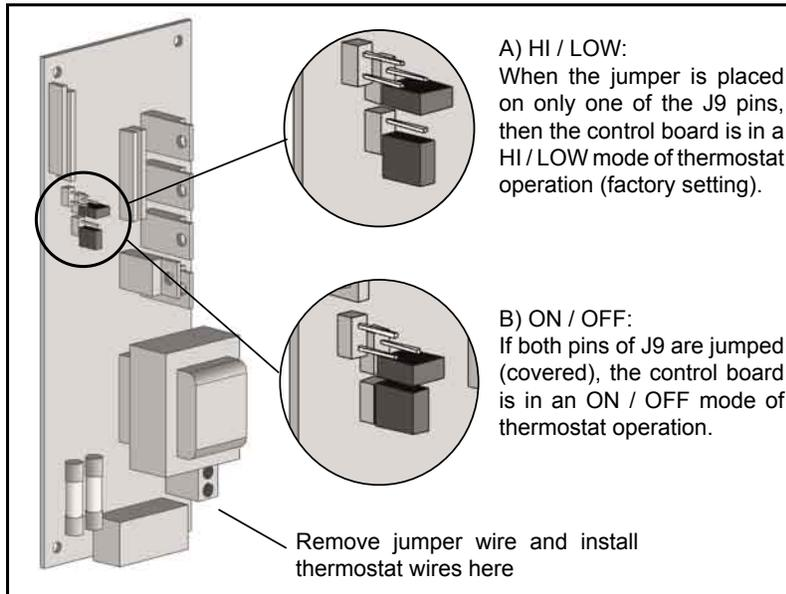
Figure 23: Circuit Board.
