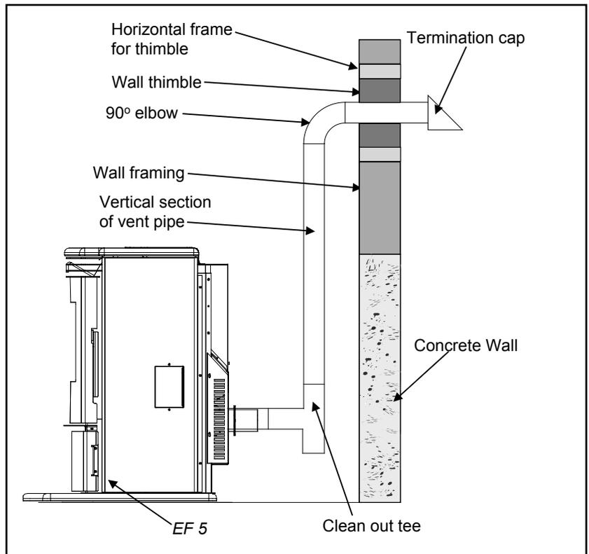
Figure 13: Venting with concrete wall behind unit .
