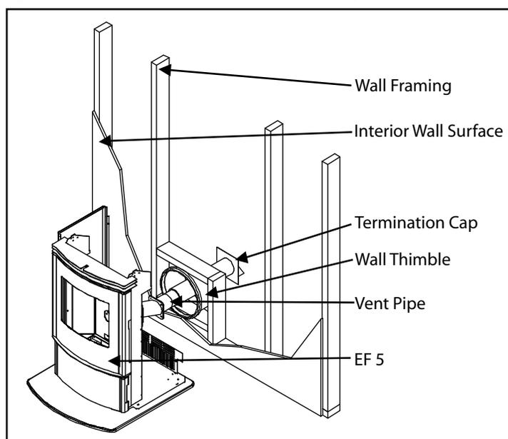
Figure 11: Straight through wall Installation.
