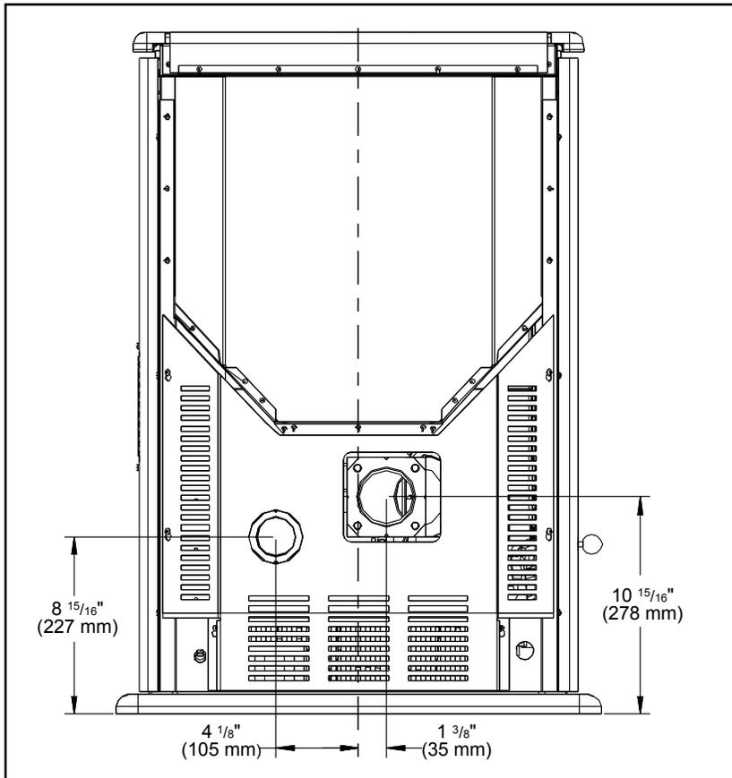
Figure 8: EF5 Inlet and Outlet Location.
