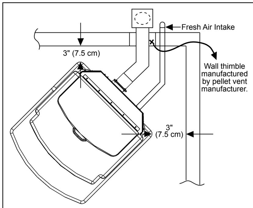
Figure 10: Corner Installation.
