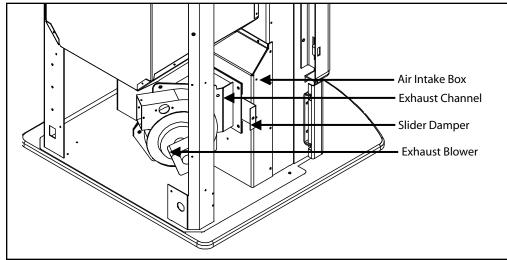
The slider damper is located behind the left side panel. To open the left side panel, undo the one screw located in the upper front corner of the cabinet side between the louvers. Also loosen three screws down the back of the side panel.
