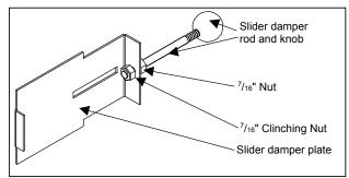
Figure 24: Slider/Damper Assembly.
