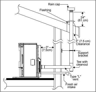
Figure 15: Outside Vertical Installation.
