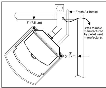
Figure 10: Corner Installation.
