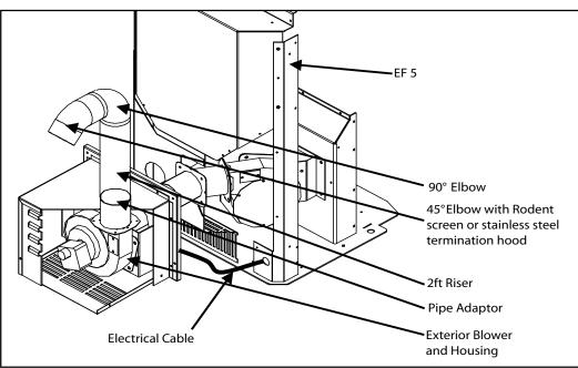
Figure 20: Through Wall Installation with Exterior Blower Kit.
