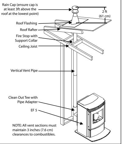
Figure 14: Inside Vertical Installation.
