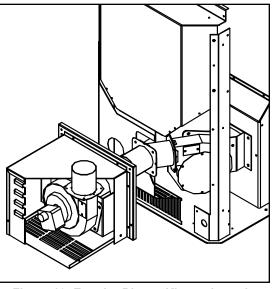
Figure 19: Exterior Blower Kit cut-through.
