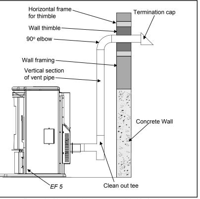
Figure 13: Venting with concrete wall behind unit .
