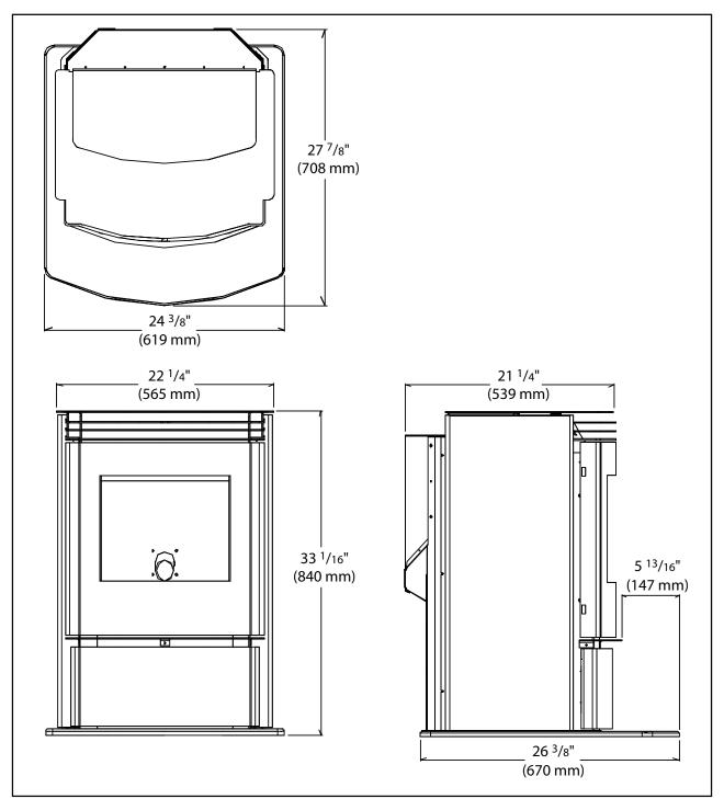
Figure 2: Dimensions of EF5.
