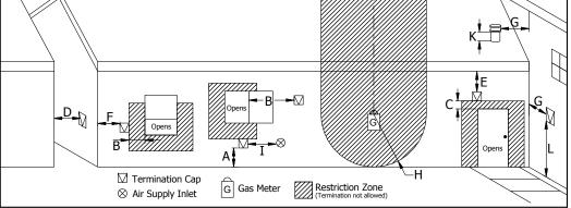
that can build up Figure 6: Use in conjunction with Table 1 for allowable exterior vent termination locations.
