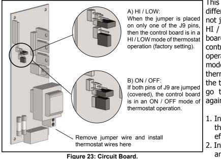
This control board can be placed into two different modes: When the jumper J9 is not jumped then the control board is in a HI / LOW mode operation. If the control board is placed with J9 jumped then the control board is in a ON / OFF mode of operation. In the ON /OFF thermostat mode, the unit will shut OFF when the thermostat is not calling for heat. When the thermostat calls for heat, the unit will go through an ignition sequence once again and relight.
