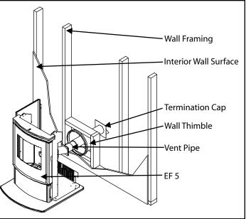
Figure 11: Straight through wall Installation.
