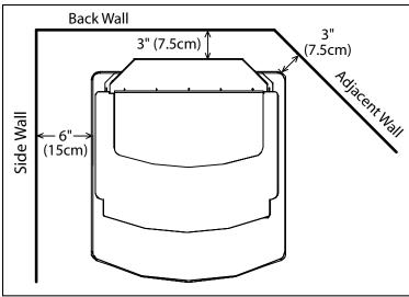
Figure 3: EF5 Clearance to Combustibles.
