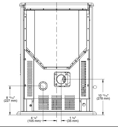
Figure 8: EF5 Inlet and Outlet Location.
