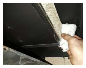
2. Grab both edges of the combustor and work it out by pulling back and forth on both sides.
