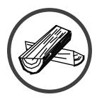
This fireplace was designed to burn solid wood fuel only (cord wood). Never use treated wood, wax logs, coal, garbage, or other materials. These materials will void the safety listing and may damage the combustor.
