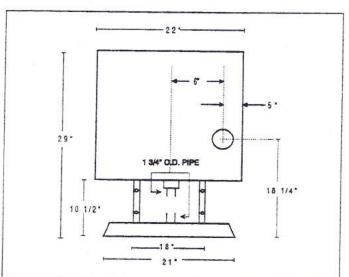
P75-F - Back View / Combustion (Exhaust) Outlet
