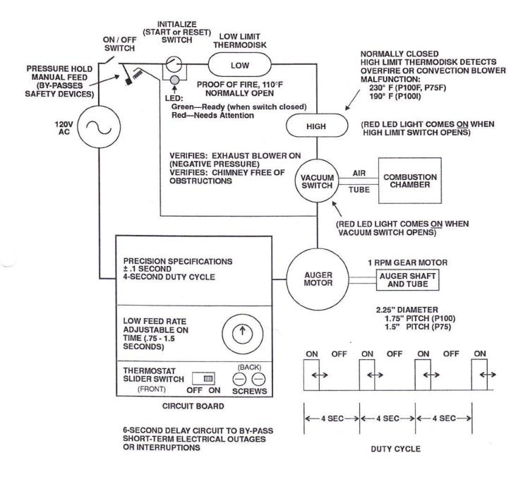
**INITIALIZE (START** or **RESET) BUTTON:** Normally closed (after activation); open (red LED light on) when high limit switch opens <u>or</u> vacuum switch opens. Red light also on when stove is in by-pass mode.
