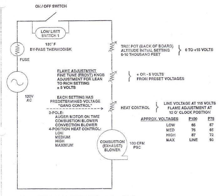
PSC means PERMANENT SPLIT CAPACITOR motor (very efficient).
