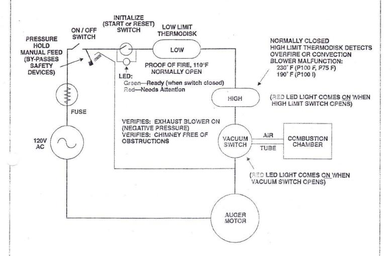
INITIALIZE (START or RESET) BUTTON: Normally closed (after activation); open (red LED light on) when high limit switch opens or vacuum switch opens. Red light also on when stove is in by-pass mode.
