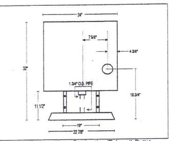
P100-F - Back View - Combustion (Exhaust) Outlet
