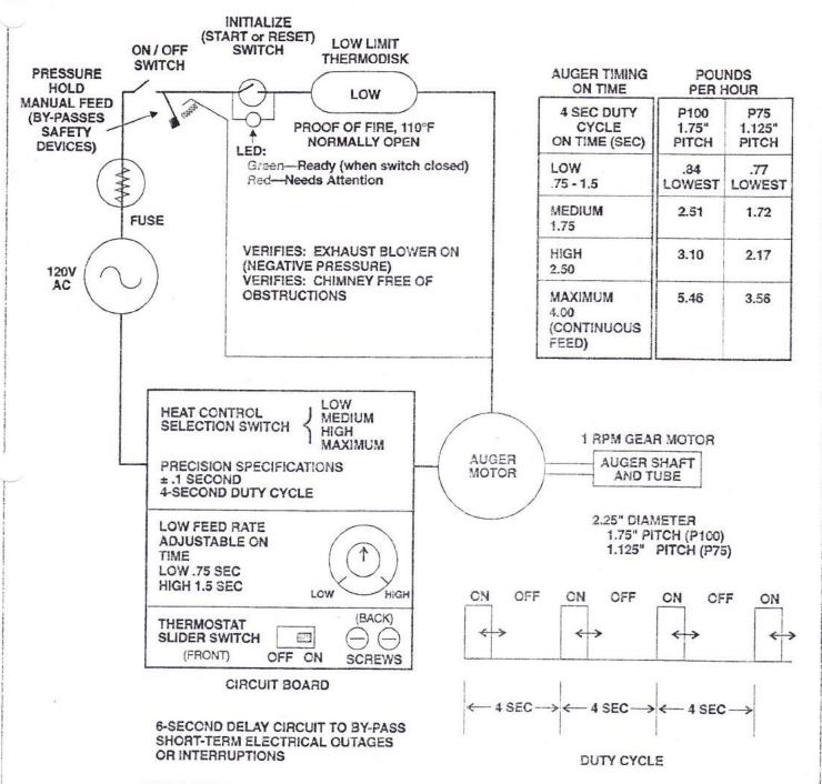
INITIALIZE (START or RESET) BUTTON: Normally closed (after activation); open (red LED light on) when high limit switch opens or vacuum switch opens. Red light also on when stove is in by-pass mode.
