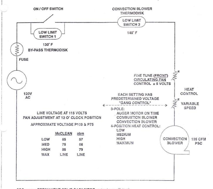
PSC means PERMANENT SPLIT CAPACITOR motor (very efficient).
