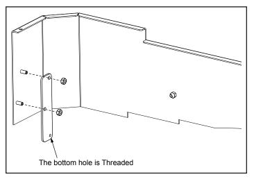
Next, install the top panel by inserting the four (4) studs through the holes in the fin on the insert. Secure with the provided nuts and a 11/32" nut driver.
