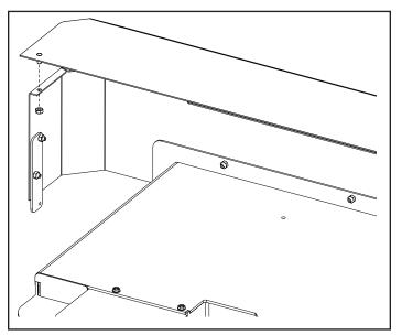
Install the side panels as shown below using (2) buttonhead screws at the top, and (1) self-tapping (Tek) screw at the bottom.
