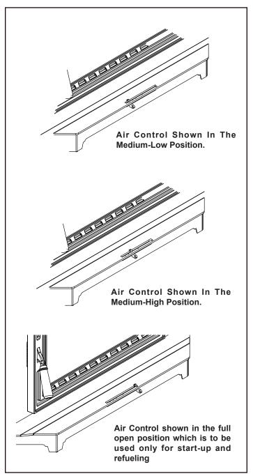
**Medium-High Burn Rate** - air control set between the second and third notch. This setting may be used to burn wood that is damp in order to keep it burning, but will consume seasoned, dry wood very fast.
