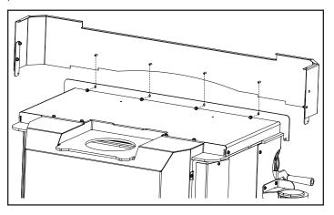
Place the top cap down onto the top, aligning the two (2) studs with the holes in the top panel. Secure from underneath with two (2) nuts.
