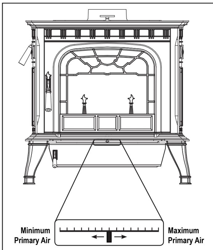
The air control lever is located directly below the load door. Sliding this lever allows you to vary the amount of air to the fire, creating a range of heat outputs. The lowest heat output setting is to the left, and the highest is to the right. The notches are provided as a reference for your comfortable heat settings. Do not, under any circumstances, alter the configuration or operation of the air control lever.
