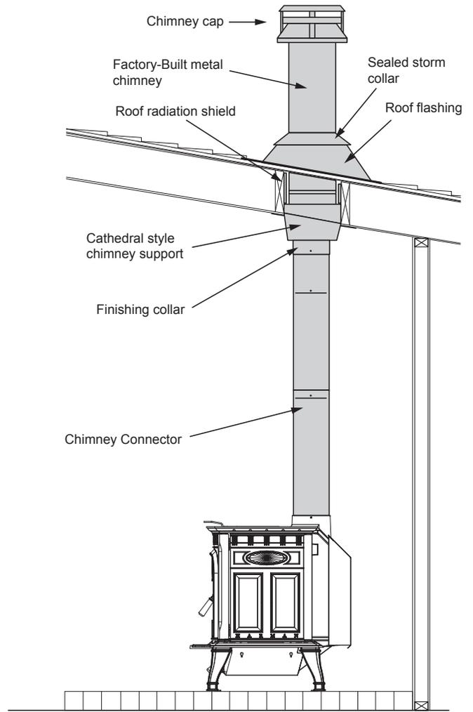
**The Chimney Connector Shall Not Pass Through an Attic or Roof Space, Closet or Similar Concealed Space, a Floor or Ceiling.**
