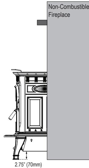
If the fireplace floor can hold the 500 lb. (250 kg) Oakwood, the stove should only be placed into the fireplace opening to the point that operation of the damper bypass control and the top load door operation is not compromised or unsafe. (See above illustration.)
