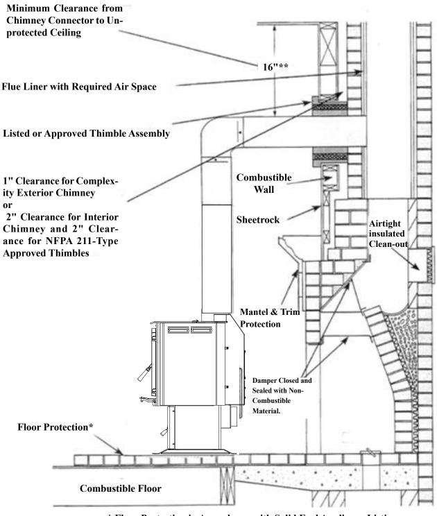
\* Floor Protection in Accordance with Solid Fuel Appliance Listing \*\* Check with your local building codes for clearance.
