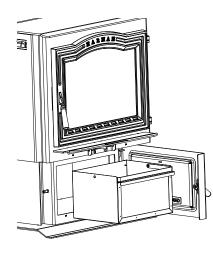
damper. Wearing heavy protective gloves, open the ash door and remove the ash pan by pulling it forward by the handle. Close the ash door and damper bypass before taking the ashes outside for safe disposal.
