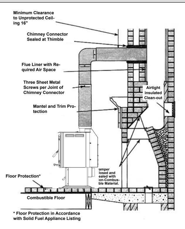
The Chimney Connector Shall Not Pass Through an Attic or Roof Space, Closet or Similar Concealed Space, a Floor or Ceiling.
