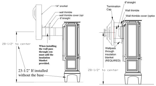
Figure 7: Components of a typical snorkel installation
