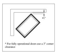
Figure 2: Clearance to combustibles
