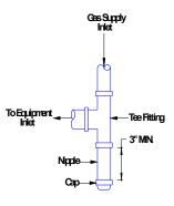
Figure 11: Typical Sediment Trap (Required in all installations)
