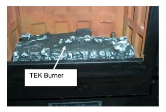
5) Place the Rear Log (1) in the firebox, on the ember burner. On the underside of the log there is a cutout that allows the pilot flame to reach the front burner under the log. Align the log in the appropriate position. It should sit as shown in the image below:
