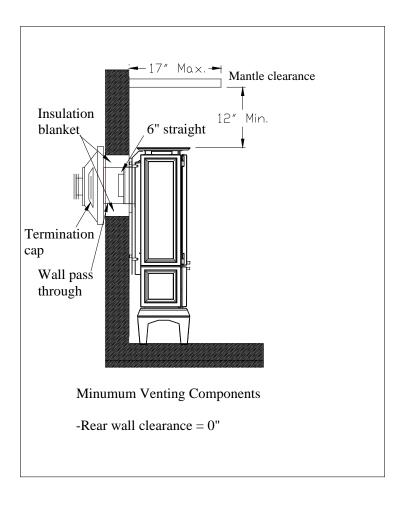
Figure 3: Minimum vent clearances
