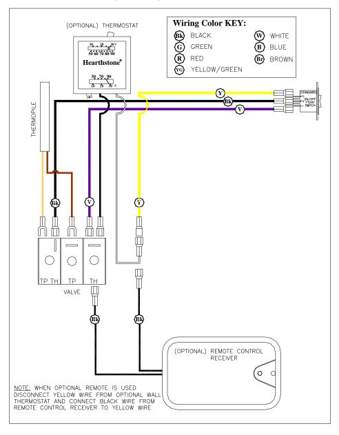
Figure 9: Wiring diagram
