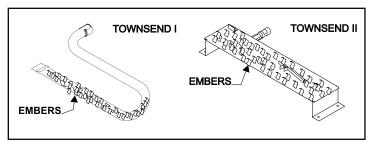
Figure 27. Placement of the Ember Material
