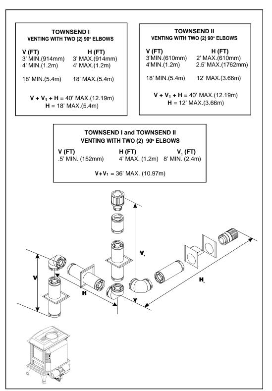
Figure 9. Vent System with Two 90° Elbows
