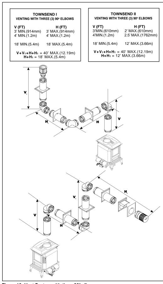
Figure 10. Vent System with three 90° elbows
