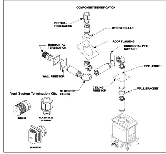
Figure 4. Vent Components and Terminations
