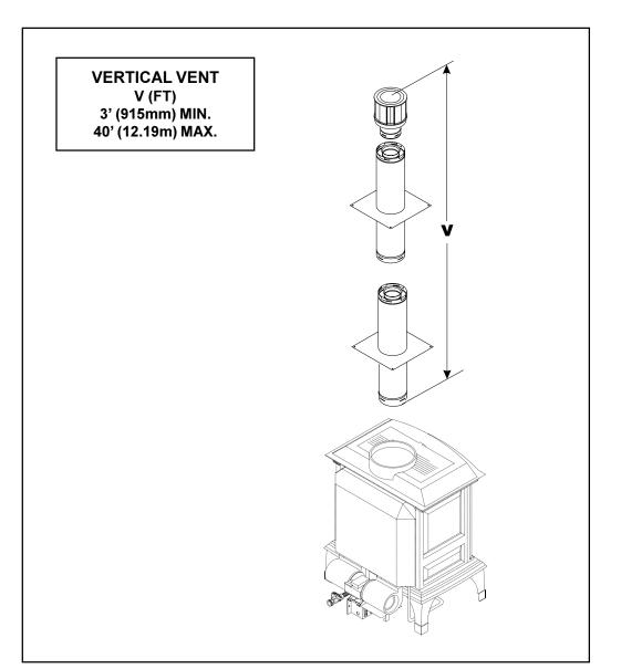
Figure 7. Straight Vertical Vent System
