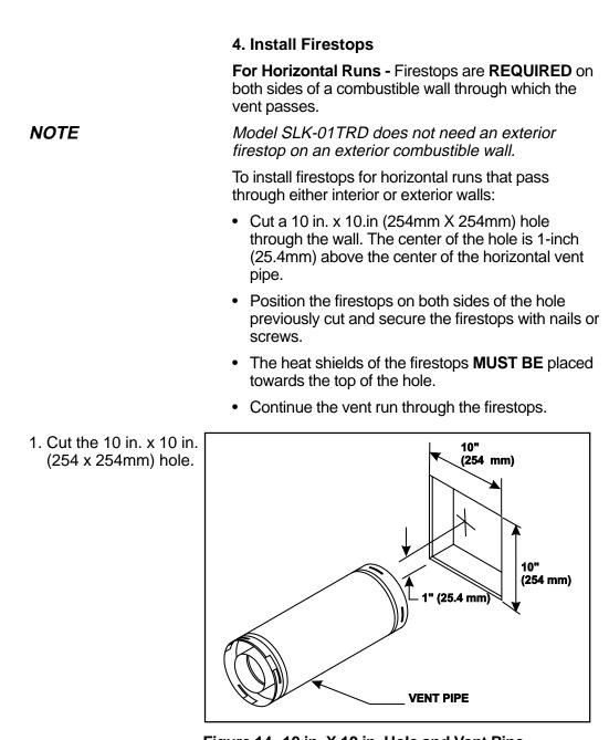
Figure 14. 10 in. X 10 in. Hole and Vent Pipe
