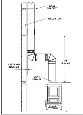
Figure 13. Installing Support Brackets
