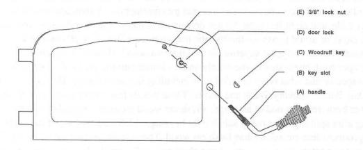
Step 1: Using a counter-clockwise motion, thread the handle(item A), into the door until tight. Then loosen the handle by approx. four turns.
