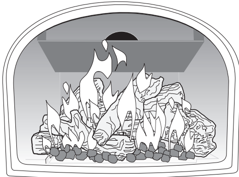
Figure 29. Flame appearance on the “high” setting after approximately 15 to 20 minutes burning.
