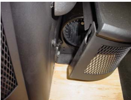
Figure 15—The ash lip and shroud are held in place by a keyhole slot and bolt system. Lifting up on the ash lip allows the bolt head to slip through the key hole.
