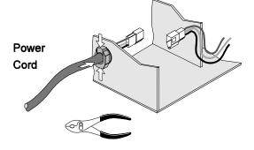
Re-attach the strain relief to the left side (use pliers to compress the strain relief from the top and bottom while pushing it into the hole).
