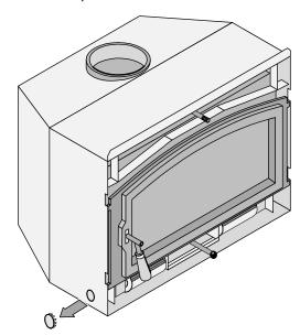
Attach the molex connector on the power cord to the molex connector on the left side of the insert.
