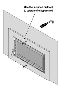
Bypass Pulled Out Used for starting and re-loading
