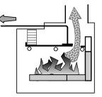
Bypass Pushed In Used for normal operation
