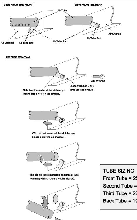
Pivot the air tube downwards and slide it out of the air channel on the opposite side.
