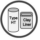
This appliance must be connected to a listed high temperature (UL 103 HT) residential type chimney or an approved masonry chimney with a standard clay tile, or stainless steel liner.
