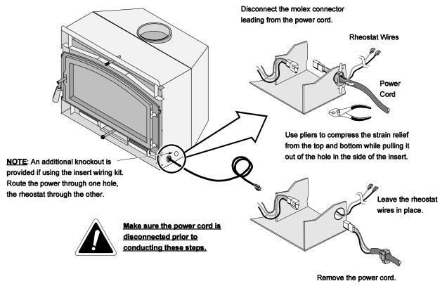
• Connect the power cord to the left side following the directions below.
