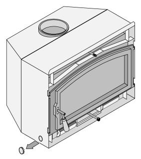
power cord to the molex connector on the left side of the insert.
