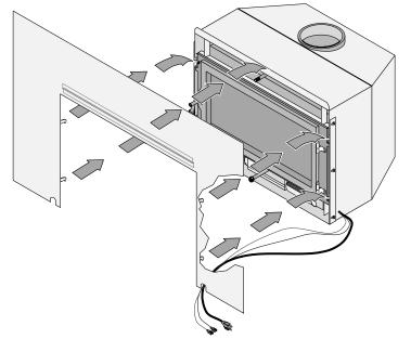
HINT: When installing the panel, route the wires through the notch on the bottom of the panel (either side).
