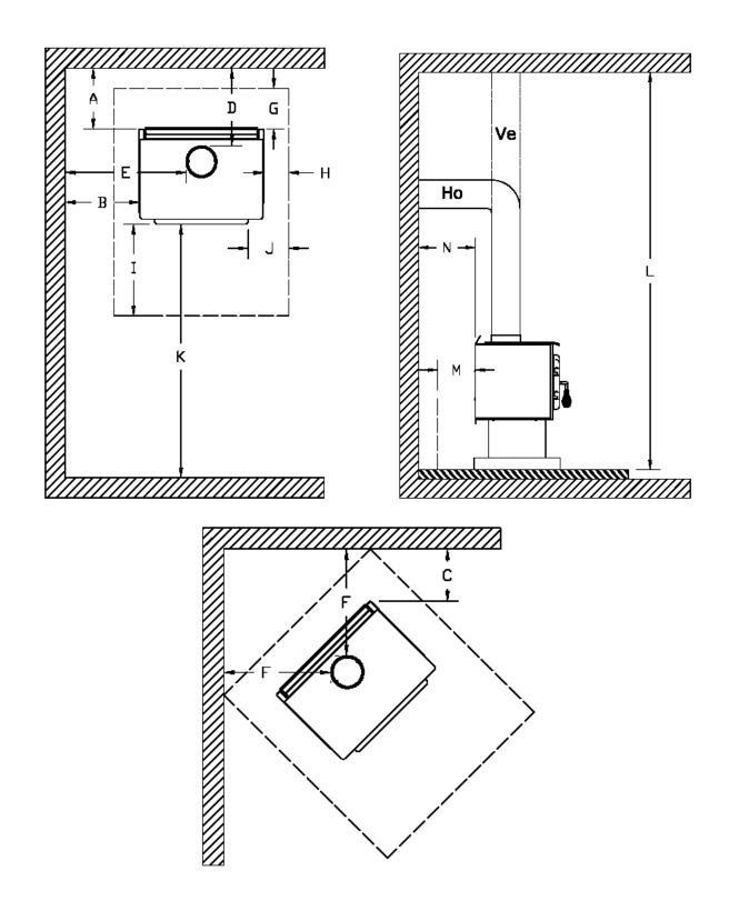
FIGURE 1.1 Clearances to combustible materials and floor protection
