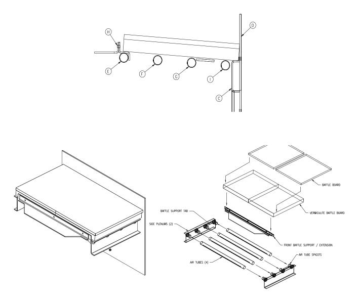
FIGURE 9 – Baffle installation & removal
