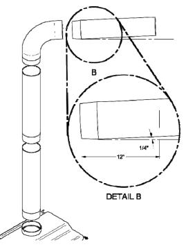
FIGURE 2.1 (B) Minimum Slope
