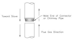
FIGURE 2.1 (A) Connecting Sections
