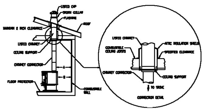
FIGURE 4 Connection to a Factory Built Chimney (Interior Shown)
