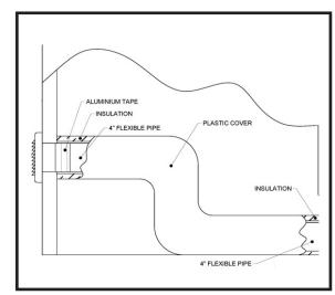
Figure 14: Typical outside air installation.
