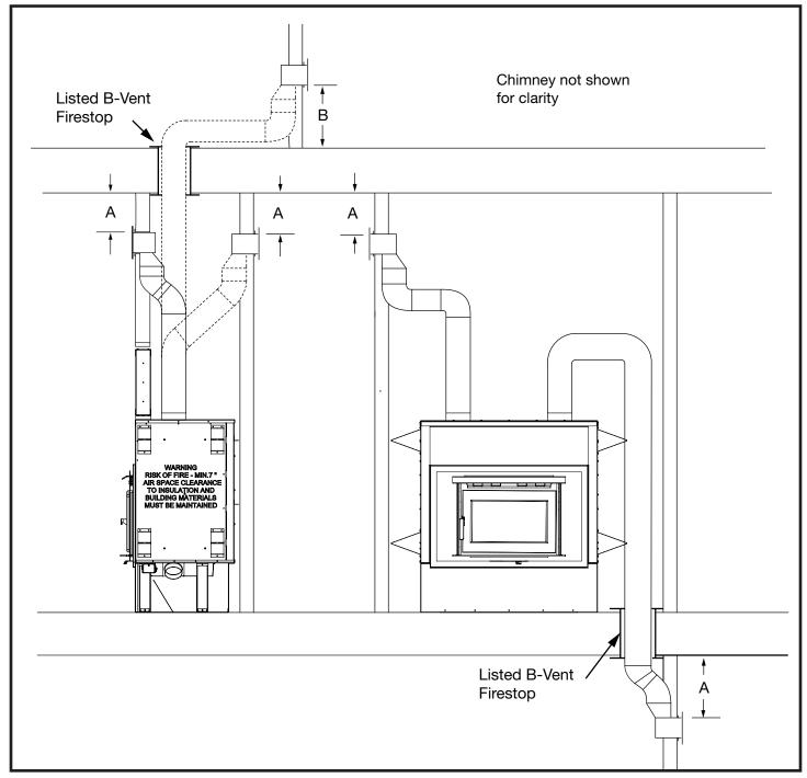
Figure 19: FP25 Remote heat duct Options.
