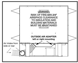
Figure 13: FP25 Air intake - rear view.
