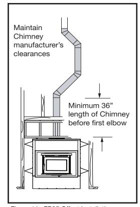
Figure 11: FP25 Offset Installation.
