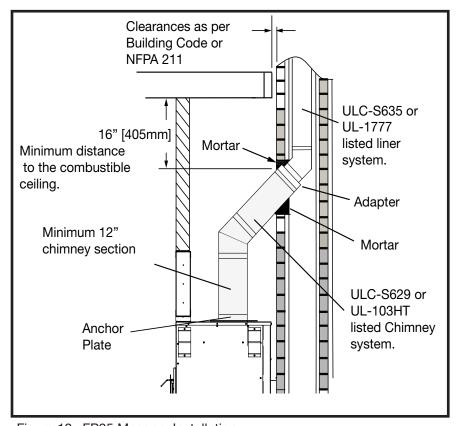
Figure 12: FP25 Masonry Installation.
