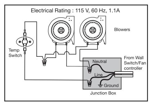
Figure 16: FP Wiring Diagraml.
