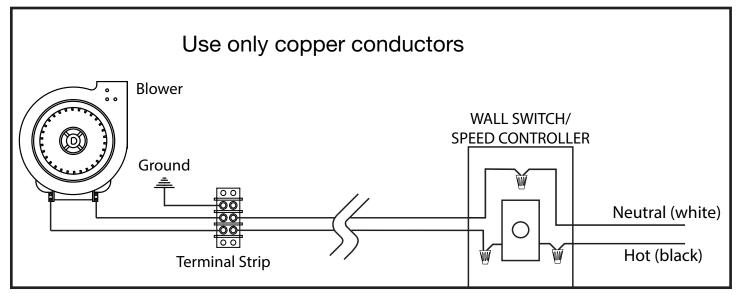
Figure 27: T120-WODC remote heat kit wiring diagram.
