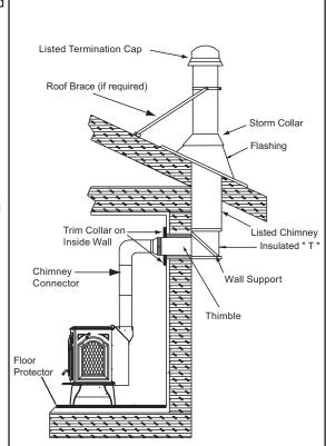
Figure 8.2 Exterior Prefabricated Chimney
