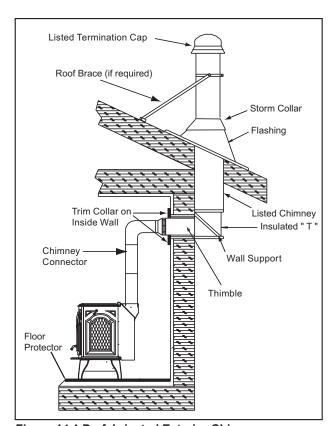
Figure 14.1 Prefabricated Exterior Chimney
