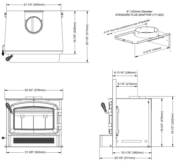
Regency Inserts are designed to use either a 5.5" (140mm) or 6" (152mm) flue.
