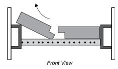
Important: push both baffle bricks so they are tight against the side walls and to the back.
