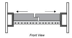
Note: When getting the chimney cleaned, remove the baffle bricks for access to the flue, then replace them when cleaning is completed.
