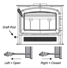
As well as a primary and glass wash air system, the unit has a full secondary draft system that allows air to the induction ports at the top of the firebox, just below the flue baffle.
