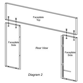
If the insert is going to sit on the hearth proceed to "Faceplate Trim Installation" (step 8) otherwise continue on to "Bottom Faceplate Installation" (step 4).
