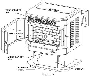
2. Remove ash buildup under the grate bottom daily or as frequently as needed. Clean the ashes out from under the burn pot by pulling the Ash Cleanout Rod in and out several times (see Fig. 6) Use the Rod Pull Tool with the Ash Cleanout Rod. This tool is hanging on a screw on the back of the stove; this provides a convenient location to keep the tool in reach and prevent it from getting lost.
