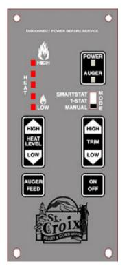
To change the Program the Stove must be in the OFF position, the unit must be completely cooled down so the Proof of Fire Switch is Open and the Thermostat slide switch must be in the Manual mode. (*See figure 3*)
