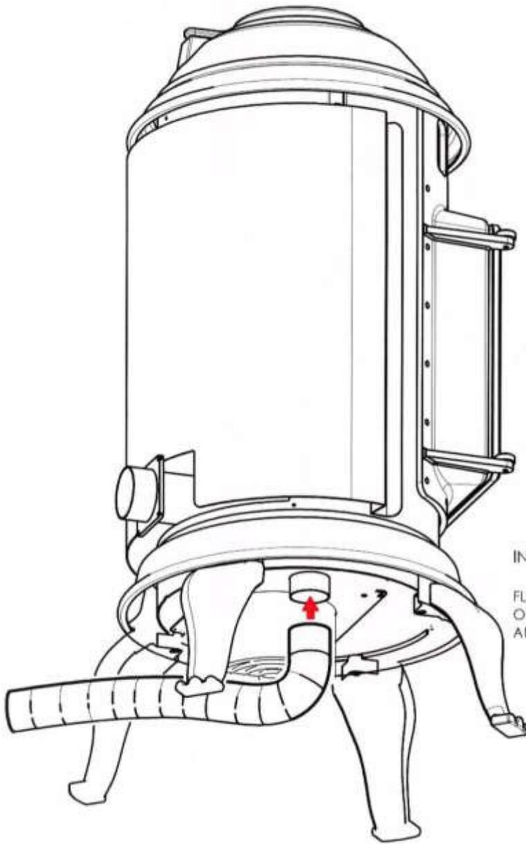
INSTALLING THE OUTSIDE AIR INTAKE TUBE.
