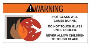
**DO NOT CLEAN GLASS WHEN HOT!** Clean the glass after the first 10 hours of operation with a recommended appliance glass cleaner. Thereafter clean as required.
