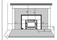
POUR INSTALLATION ET UTILISATION CONFORMÉMENT AUX INSTRUCTIONS DU FABRICANT ET AUX CODES LOCAUX DU BÂTIMENT. HAUTEUR DE PLAFOND MINIMAL: 7PI (2,13m).
