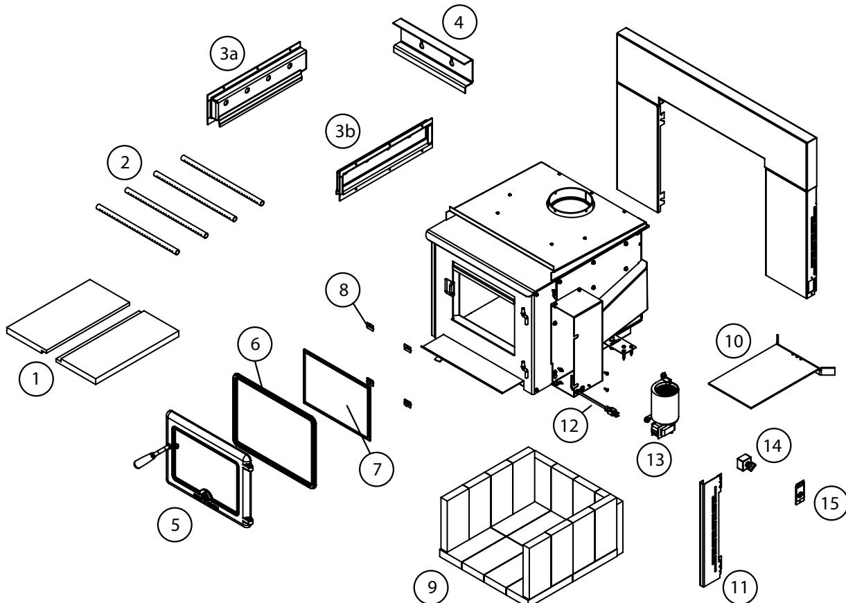
Figure23:TN20B INS Exploded Parts View.
