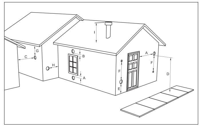
FIGURE 5 VENT TERMINATION CLEARANCES
