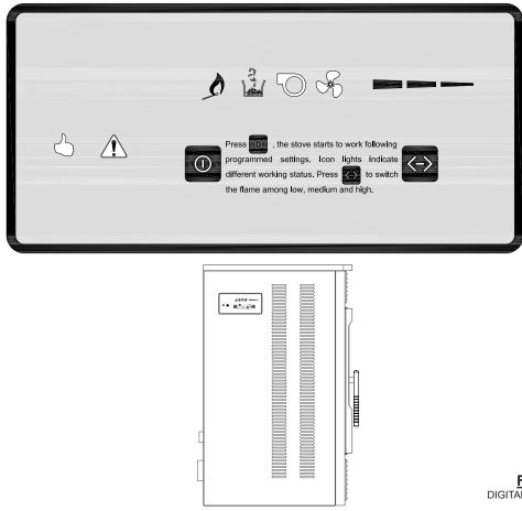
FIGURE 9 DIGITAL CONTROL PANEL
