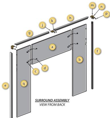
1. Lay pieces face down on carpet or other soft surface to protect finish during assembly. The Surround consists of two side panels, a top panel, and a decorative trim frame.
