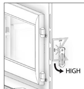
After the first high burn load and the stove is well warmed up, adjust the unit as needed for a medium or low burn setting.
