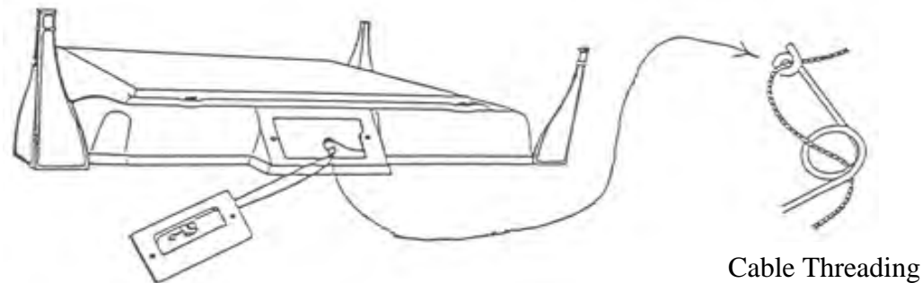
Fig. A-2 Primary Air Regulator System Ready to be Installed
