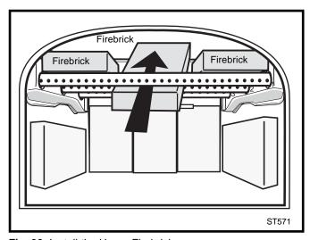
Fig. 30 Install the Upper Firebricks.
