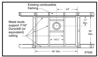
Fig. 25 Reflected ceiling plan.
