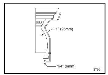
Fig. 21 A custom-formed mantel shield.
