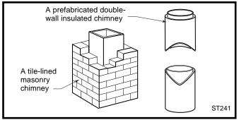
Fig. 3 Standard Chimney Types
