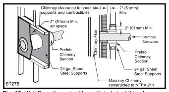
Fig. 12 Wall Pass-through with ventilated steel thimble.
