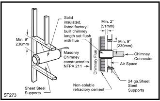
Fig. 10 Wall Pass-through using factory-built insulated chimney section.
