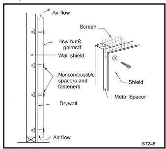
Fig. 16 Approved Wall shield construction
