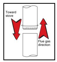
Fig. 4. Chimney connector.
