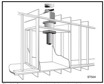
Fig. 24 Cutaway perspective of alcove installation.
