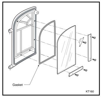
Fig. 35 Door glass installation.
