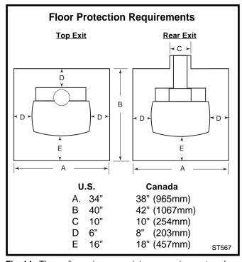
**Fig. 14** These dimensions are minimum requirements only. Use greater dimensions whenever possible.
