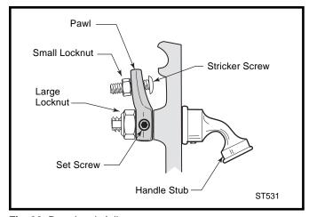
Fig. 36 Door Latch Adjustment
