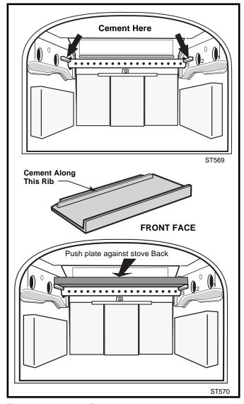
Fig. 29 Installing the Smokeshelf.
