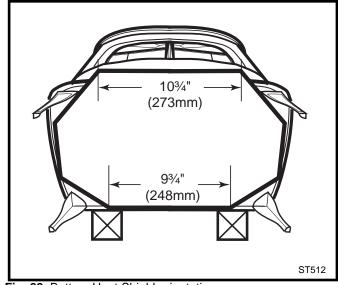
Fig. 28 Bottom Heat Shield orientation.
