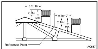
Fig. 2 The 2'-3'-10' Chimney Rule.
