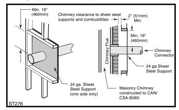
Fig. 13 CSA approved Wall Pass-through.
