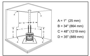
**Figure 23** - Corner installation, vertical chimney connector, with rear, stove, connector and wall shields. Wall shields **MUST** meet at corner. Connector heat shield extends 28" (710mm) above flue collar. A 24" (610mm) diameter ceiling heat shield must surround the chimney and be suspended 1" (25mm) from ceiling.
