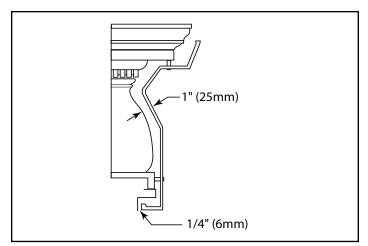
Figure 14 - A custom-formed mantel shield.
