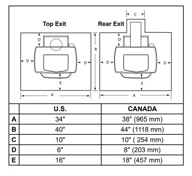
In Canada, the floor protector required under the stove must extend 18" (460 mm) to the front (labeled 'E', Figure 11), and 8" (203 mm) from the sides and rear. ('D', Figure 11)
