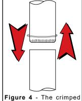
**Figure 4** - The crimped end of the connector points toward stove.
