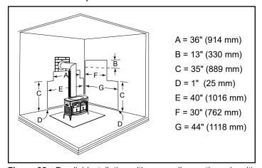
**Figure 25** - Parallel installation with rear wall pass-through, with stove, connector and wall shields. Wall shields may meet at corner. Connector heat shield extends 28" (710mm) above flue collar, or below elbow, whichever is less. Wall pass-through must comply with codes.
