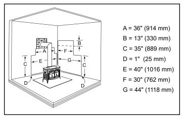
**Figure 22** - Parallel installations with rear wall pass-through, two wall shields. Reduced clearances for both rear and side walls. Wall shields may meet at corner if desired. Shielding for connector is centered behind connector. Wall pass-through must comply with codes.
