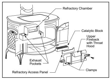
Figure 46 - Removing the catalytic element.
