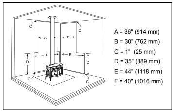
**Figure 21** - Parallel installation, vertical chimney connector, two wall shields. Reduced clearances for both rear and side walls. Wall shields may meet at corner if desired. Shielding for connector is centered behind connector.
