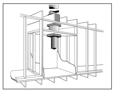
Figure 18 - Cutaway perspective of alcove installation.
