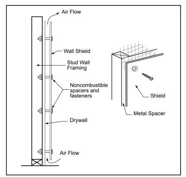
Figure 13 - Approved wall shield construction.
