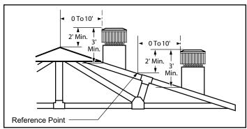
Figure 3 - The 2'-3'-10' Chimney Rule.
