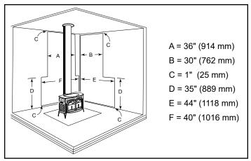
**Figure 24** - Parallel installation, vertical chimney connector, with stove, connector and wall shields. Maximum reduction for rear and side walls. Wall shields may meet at corner. A heat shield 24" (610mm) in diameter suspended 1" (25mm) below the ceiling must surround the chimney.
