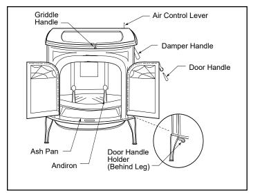
Figure 32 - The Intrepid II controls.
