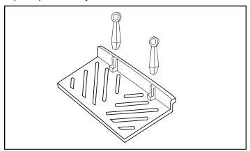
Figure 35 - Remove the andirons for front loading.
