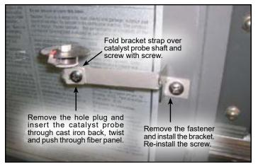
Figure 30 - Attach the temperature probe.
