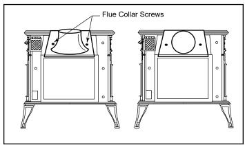
Figure 29 - Reversing the flue collar.
