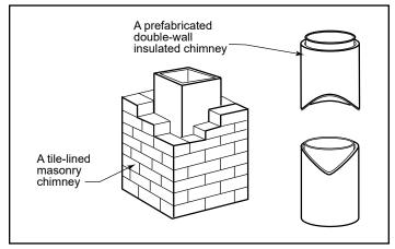
Figure 2 - Standard chimney types.
