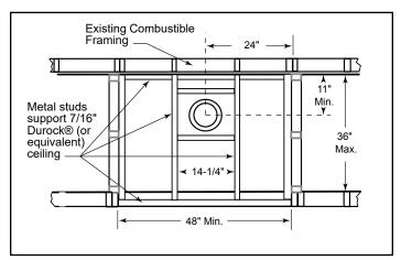
Figure 19 - Reflected ceiling plan.
