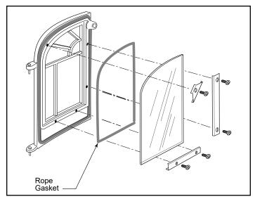
Figure 42 - Door glass installation.
