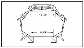
Figure 27 - Attach bottom heat shield.
