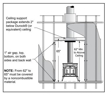
**Figure 20** Front view: 65" minimum clearance form hearth to combustibles on front face. Combustible facing may overlap metal studs by only 1". It should not extend below the height of the noncombustible ceiling.
