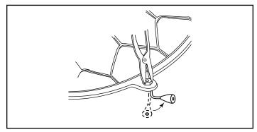
Figure 31 - Attaching the griddle handle.
