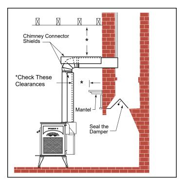
Figure 7- Chimney connector enters chimney above the fireplace.
