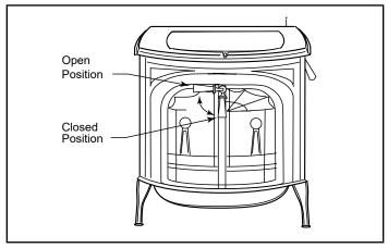
Figure 37 - To open the front doors, turn handle clockwise.
