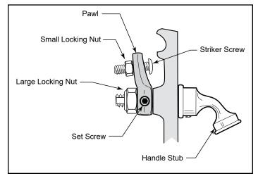
**Figure 44 -** Turn the door latch striker screw in or out to tighten or loosen the door latch.
